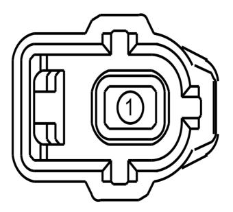
Pin Circuit GaugeCircuit FunctionQualifier1208 (GY)20Engine oil pressure switch signal
